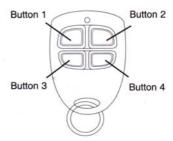
The tag key offers an alternative method of arming and disarming the alarm system; the alarm can accommodate 4 radio keys and 4 tag keys at any one time.
